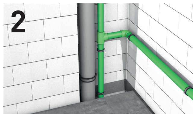
Favourable placement of the riser in the shaft
