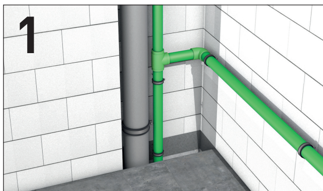
Positioning of a fixed point clamp
